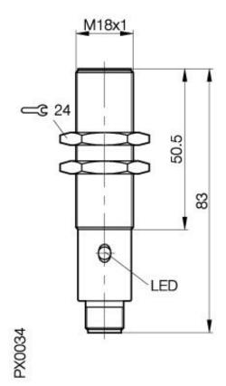
Inductive Sensors BES 516-538-S 4-H M18x1 x 83 normally-open Sn=5mm shielded
